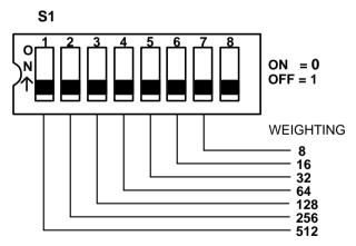
The base address calculation is as shown below.
